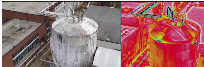
Figure 87: Use Case – Aging Facility Inspections (Insulation Loss)
