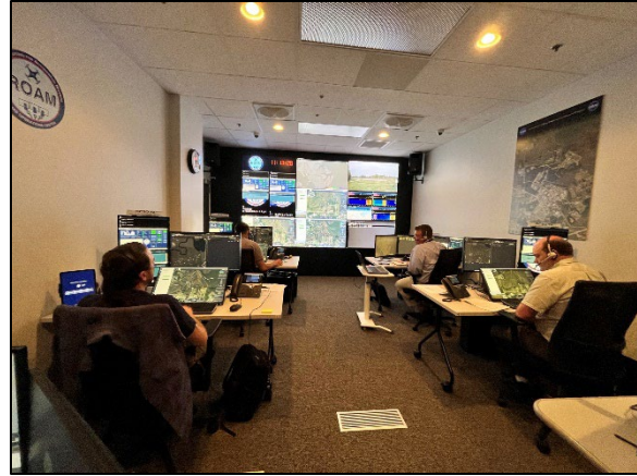
Figure 14: Six Interconnected LaRCnet Workstations / Interchangeable Based on User's Role
