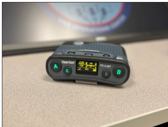
Figure 39: Clear-Com Equipment – Beltpack
