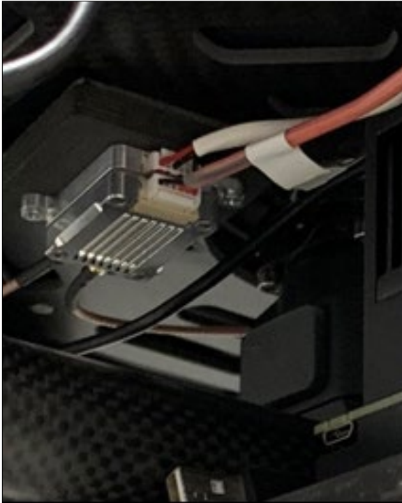
Figure 28: uAvionix microLink Radio Installed on Vehicle
