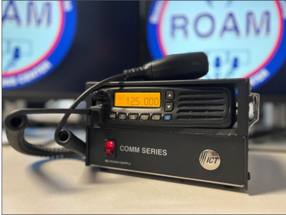
Figure 42: Over-the-Air Aeronautical Radio for Range Safety Officer in ROAM
