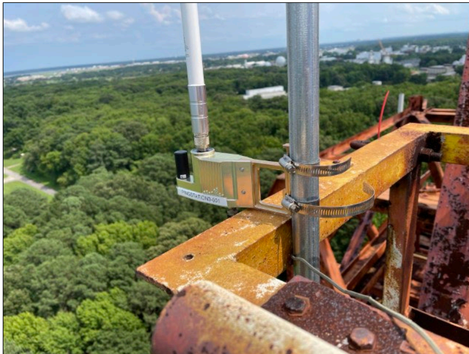
Figure 20: ADS-B Receiver at NASA’s Langley Research Center
