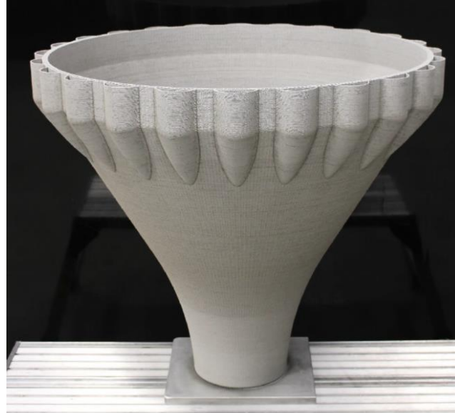
Continued RAM enhanced Aluminum L-DED for launch vehicle applications
