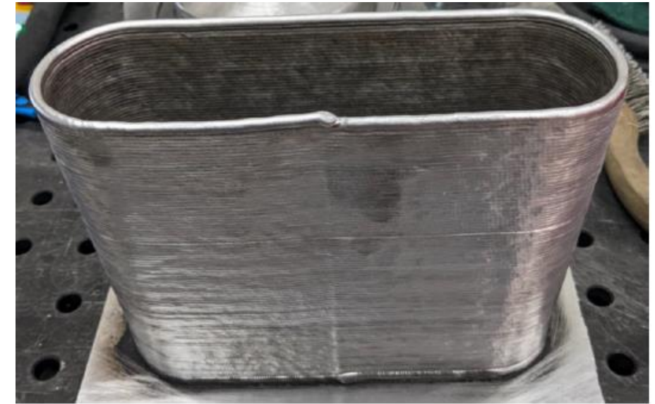
Aluminum weld wire undergoing WA-DED/WAAM testing and development
