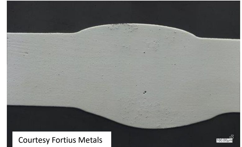
Internally produced RAM2 wire. Acceptable porosity.
