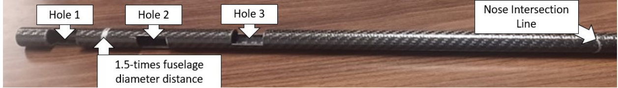
Figure 6: Picture of holes 1, 2, and 3 cut into the central boom
