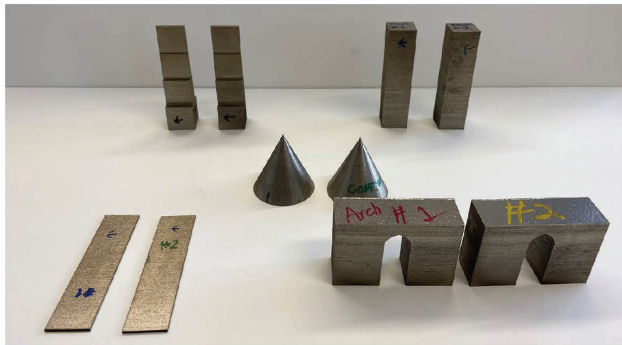
Figure 2: Final parts manufactured and cut off the build plates
