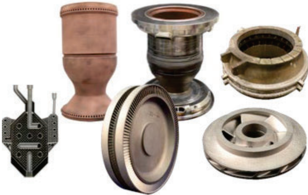
Figure 6.0-1. Examples of Engine Hardware Produced via AM [adapted from Gradl, 2022b]
