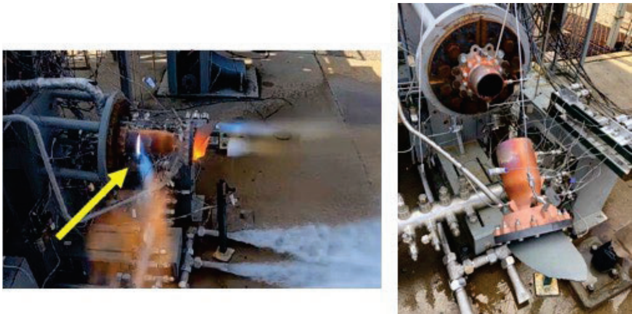
Figure 6.0-2. Test Stand Failure of AM Combustion Chamber [Gradl, 2022b]
