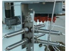
Sensor probes in emissions testing rig manifold
