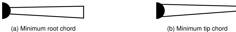
Figure 9: Proprotors designed with a linear chord distribution with a constraint on the minimum root or tip chord.
