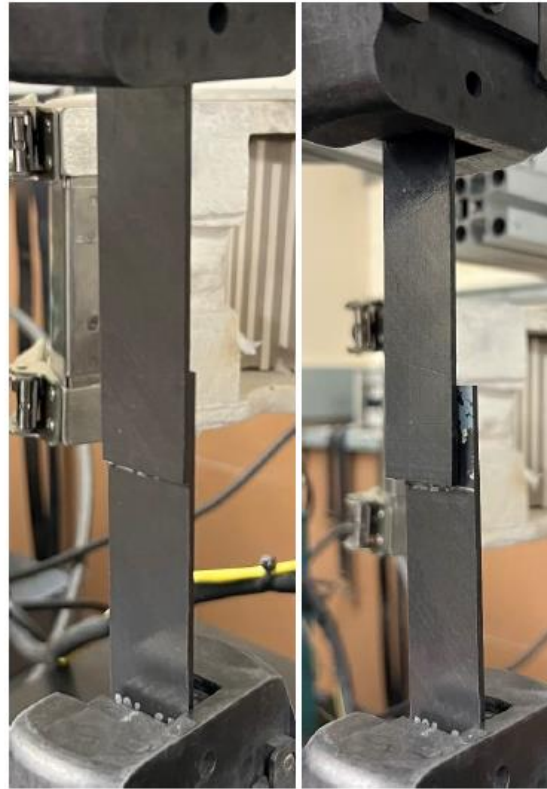
SLS test setup before (left) and after (right) failure.
