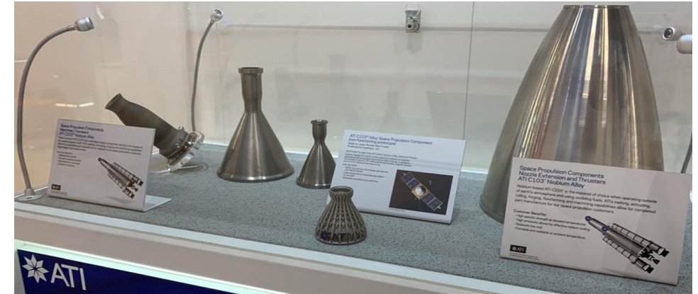
Examples of L-PBF and EBAM C103 components.
