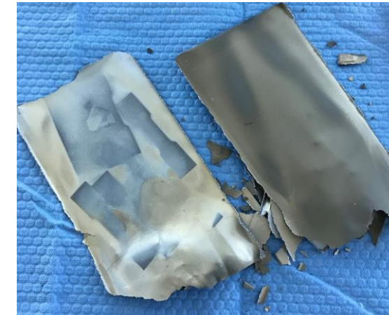
Post-HIP Ta wrap brittle from C & O [1]
