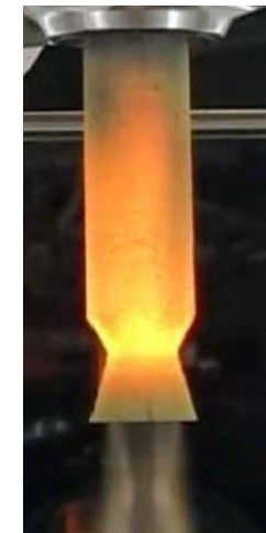
AM C103 Hot Fire Test
