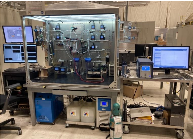
Figure 6. Test stand at MSFC housing a MFECR at EDU scale.
