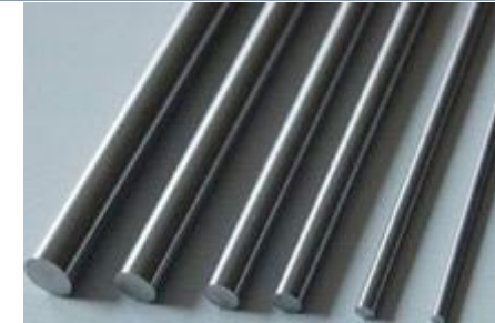
C103 forged bar stock. Courtesy ATI.
