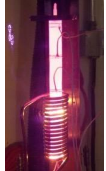
TZM alloy heat pipe. Courtesy Advanced Cooling Technologies.
