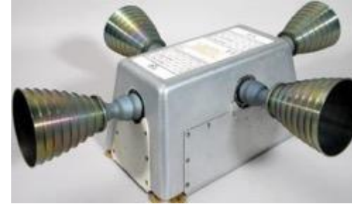
Apollo CSM RCS using C103. Courtesy Aerojet-Rocketdyne
