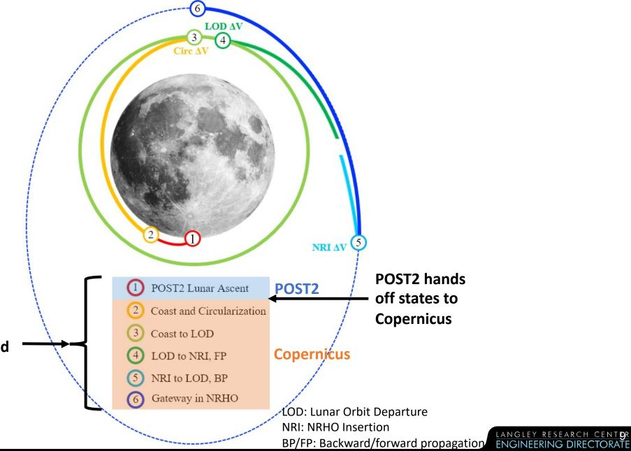
All segments of the trajectory are optimized in an end-to-end sense using SNOPT within Copernicus
