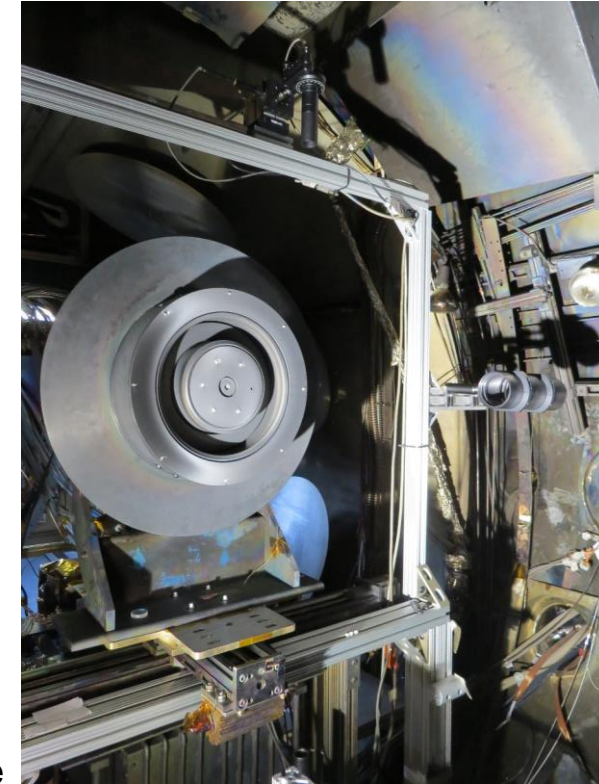
In-chamber configuration for azimuthal LIF measurements at JPL
