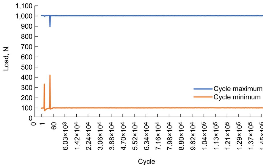
Figure 4.—Maximum and minimum load as function of cycles for practice fatigue test of YS-90A specimen with 0.75-in. nominal width. Load ratio  $R = 0.1$ ; maximum load = 1,000 N nominal; minimum load = 100 N nominal; frequency = 5 Hz; cycles to failure = 153,000.
