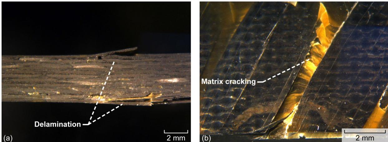
Figure 10.—Representative YSH-60A sample. (a) Side view showing delamination. (b) Tension surface view showing epoxy and carbon fiber cracking.
