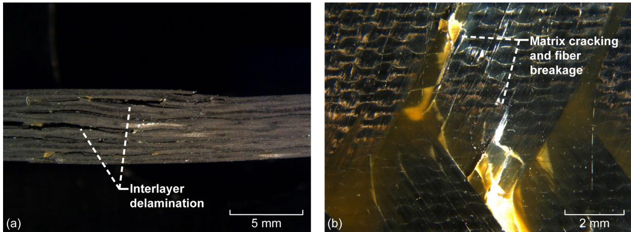
Figure 11.—Representative YS–80A fatigue sample. (a) Side view showing prominent interlayer delamination. (b) Compression surface view showing cracking within fiber tows and epoxy.
