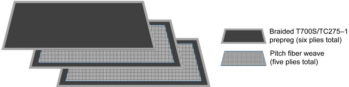
Figure 1.—Incorporation of dry pitch fiber weave into T700S/TC-275-1 prepreg (Ref. 12).
