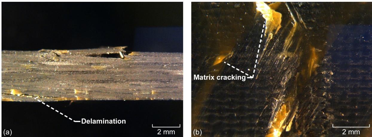
Figure 9.—Representative baseline sample after failure. (a) Side view showing delamination. (b) Compression surface view showing epoxy matrix cracking.
