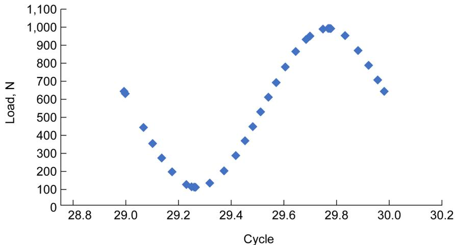
Figure 5.—Waveform of one cyclic load during fatigue testing. Load ratio  $R = 0.1$ .
