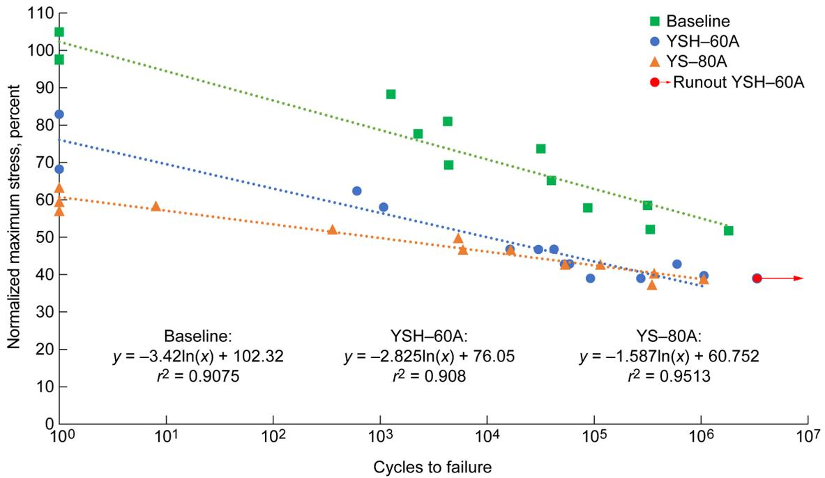
Figure 7.—Fatigue life curve, maximum stress (normalized relative to baseline) versus cycles to failure, for hybrid PAN-pitch YSH-60A, YS-80A, and baseline composite materials. Stress ratio  $R = 0.1$ ; frequency = 4 Hz; data fit to semilogarithmic trend line. The correlation coefficient  $r^2$  of best fit is provided for each line.
