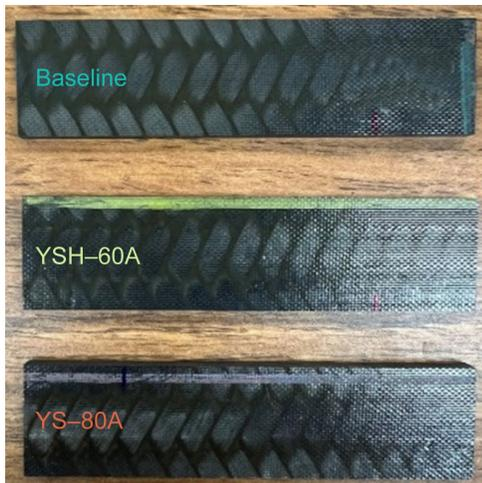
Figure 2.—Baseline, YSH-60A, and YS-80A hybrid PAN-pitch fatigue coupons received from CTL.
