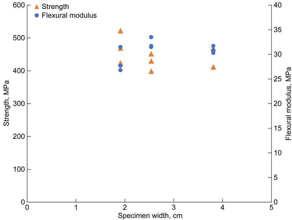
Figure 6.—Average strength and flexural modulus of practice bend specimens with YS-90A pitch-based graphite fiber interleave at nominal widths of 1.91, 2.54, and 3.81 cm.
