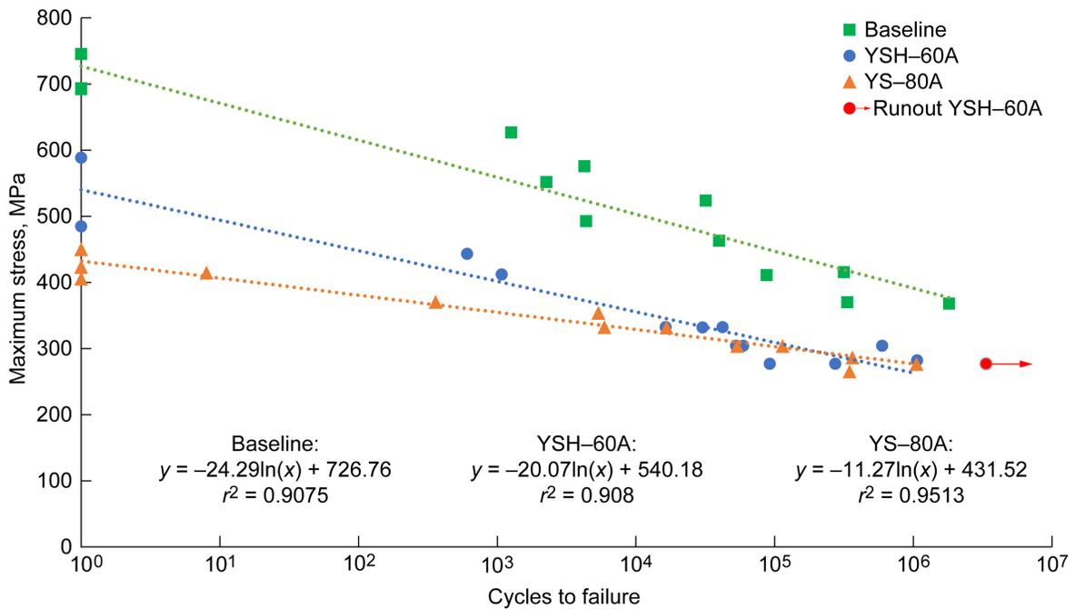
Figure 8.—Fatigue life curve, maximum stress versus cycles to failure, for hybrid PAN-pitch YSH-60A, YS-80A, and baseline composite materials. Stress ratio  $R = 0.1$ ; frequency = 4 Hz; data fit to semilogarithmic trend line.
