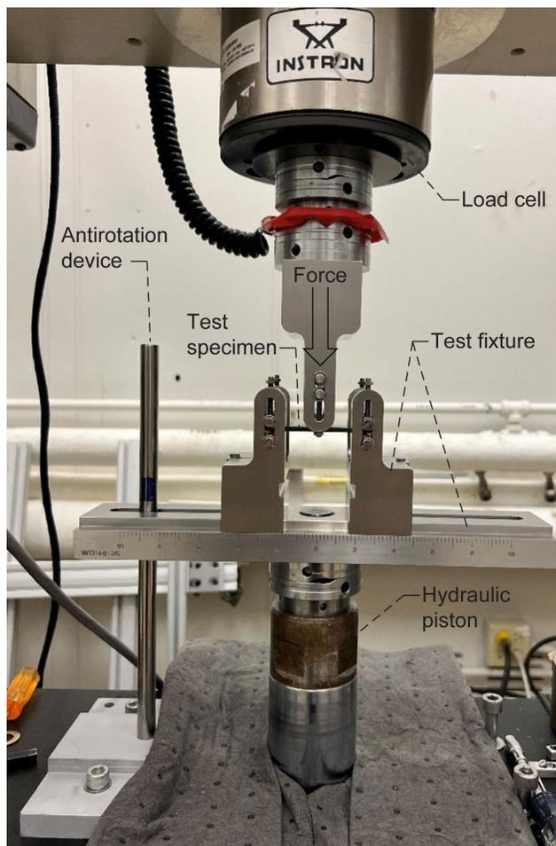
Figure 3.—Antirotation device installed on test frame to prevent flexural fatigue fixture from rotating during testing; test specimen under load with 2.5-in. span.
