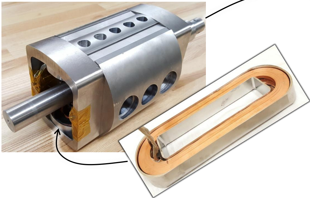
Coils under high-speed rotation (Feb '20)
