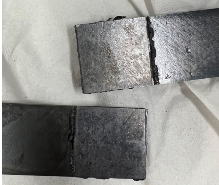
Figure 18.—Thermal degradation and flowout of PPS film in broken sample.
