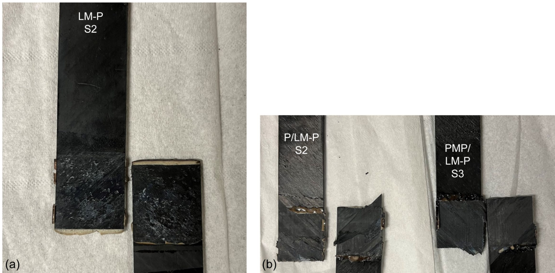
Figure 22.—Broken SLS joints using LM-PAEK interlayer at RT. (a) PEEK adherends with LM-PAEK interlayer. (b) Hybrid PEEK/LM-PAEK adherends.
