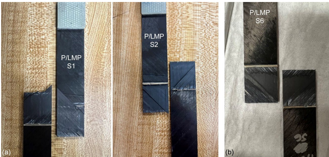
Figure 15.—Broken SLS joints using LM-PAEK interlayer with hybrid PEEK/LM-PAEK adherend. (a) At RT. (b) At ET.
