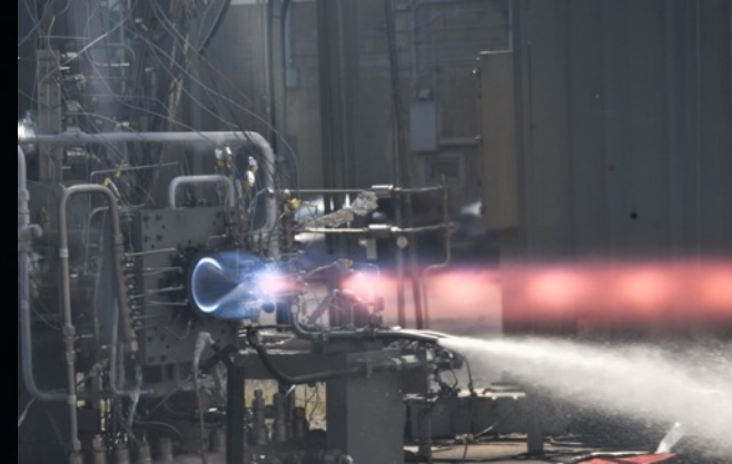
Rotating Detonation Rocket Engine (RDRE) Testing at MSFC Test Stand 115
