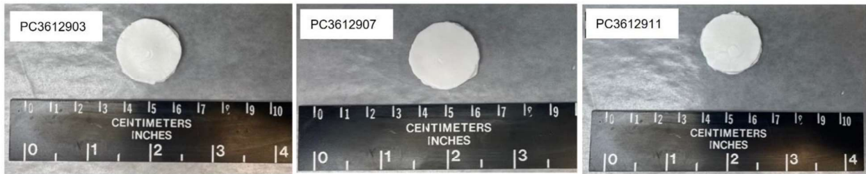
Supplementary Figure 1. BNNP foam macrographs: BNNP foam with a) parallel, b) intermediate, and c) perpendicular walls to the neutron source
