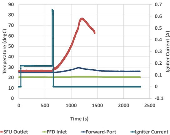
**Figure 4. Temperature results for Saffire VI-3 (two-sided PMMA).** The duct flow was reduced at 1120 s and terminated at 1420 s so the inlet and outlet traces end. The forward port sensor is the nearest to the Saffire flow duct outlet.
