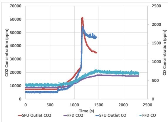
**Figure 6. CO and CO<sub>2</sub> concentrations for Saffire VI-3 (two-sided PMMA)** The duct flow terminated at 1420 s so the outlet traces end. The flow was changed from 20 cm/s to 5 cm/s at 1120 s. At this lower flow rate, the outlet CO<sub>2</sub> and CO levels increased due to the lower ambient flow. The forward port sensor is the nearest to the Saffire flow duct outlet and the zenith sensor is near the far field device.
