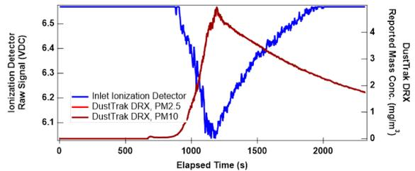
**Figure 7. Far field ionization smoke detector and particulate matter measurements for Saffire VI-3 (two-sided PMMA).**
