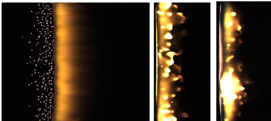
**Figure 3. Representative front-view (sample surface) images for each Saffire VI test after the flame is well established. From left: SIBAL fabric (test 2), 2-sided PMMA (test 3), and 1-sided PMMA (test 4). Oxidizer flow is from the left at 20 cm/s in all cases.**
