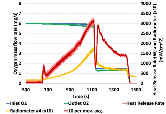
**Figure 5. Inlet and outlet oxygen concentrations for Saffire VI-3 (two-sided PMMA) with the calculated heat release based on the oxygen consumption.** The flow was changed from 20 cm/s to 5 cm/s at 1120 s and terminated at 1420 s. The dip at 1120 s is due to the impact of the transient flow change on the oxygen sampling.
