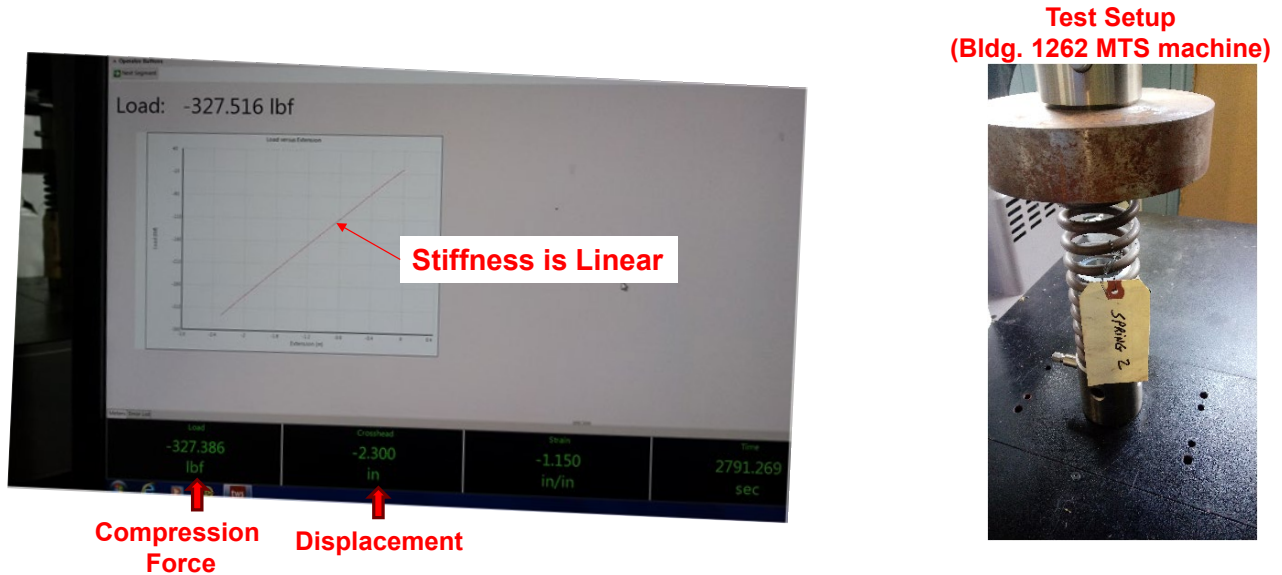
Figure 14. Compression Spring Test Results (Left); Creep Testing Setup (Right)
