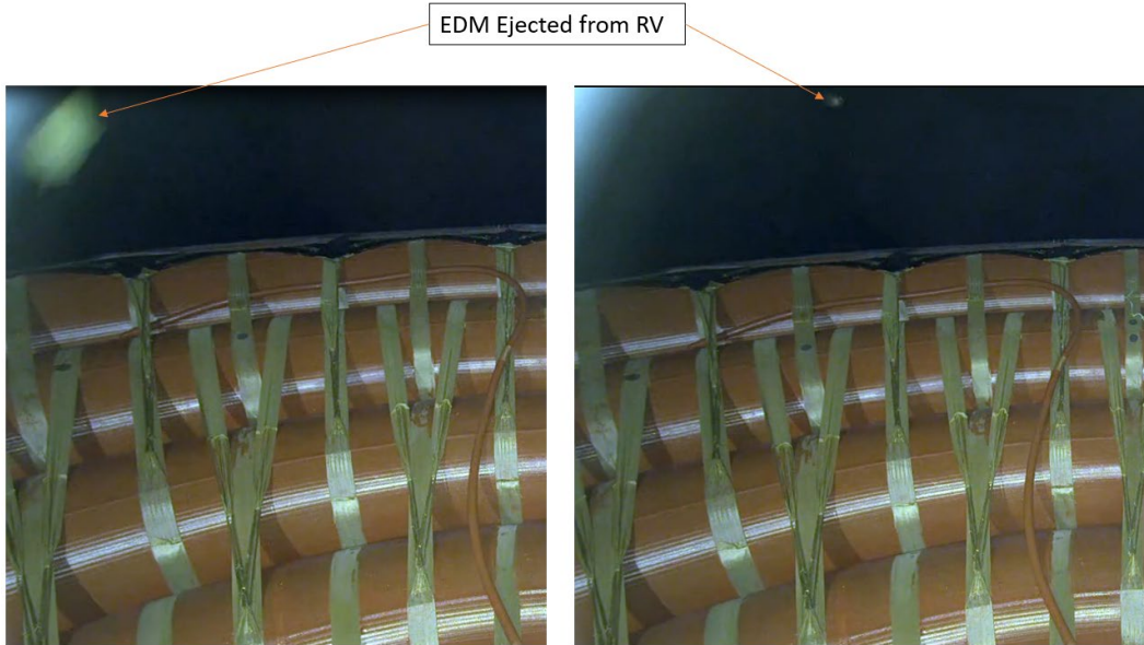
Figure 23. EDM Ejecting from RV
