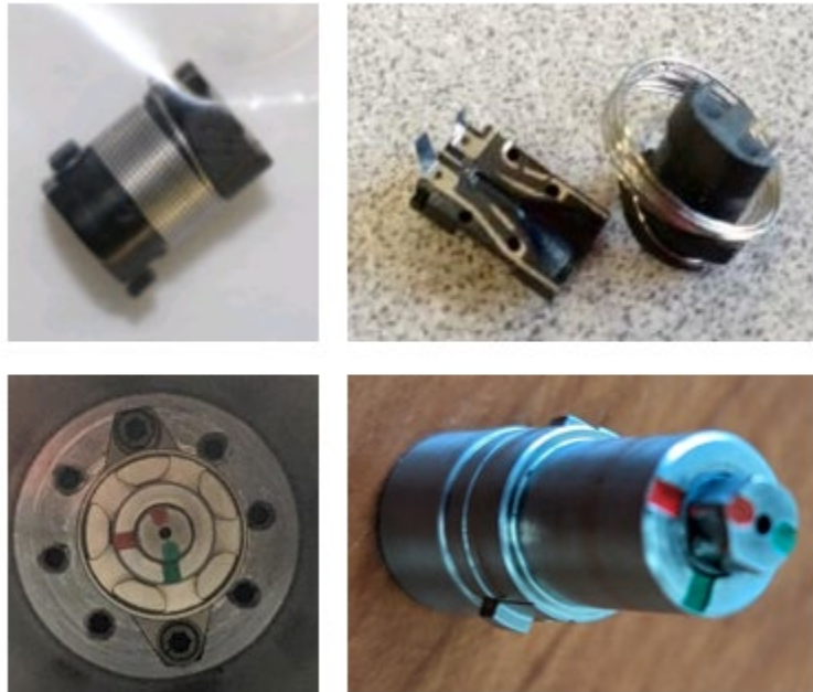
Figure 12. NEA Split Spool (Top), Mechanical Release (Bottom)
