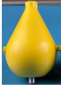
Figure 4. Ejectable Data Module
