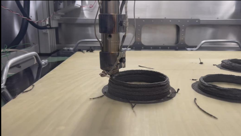
RPC is printed at 0.250 torr on a heated build plate
