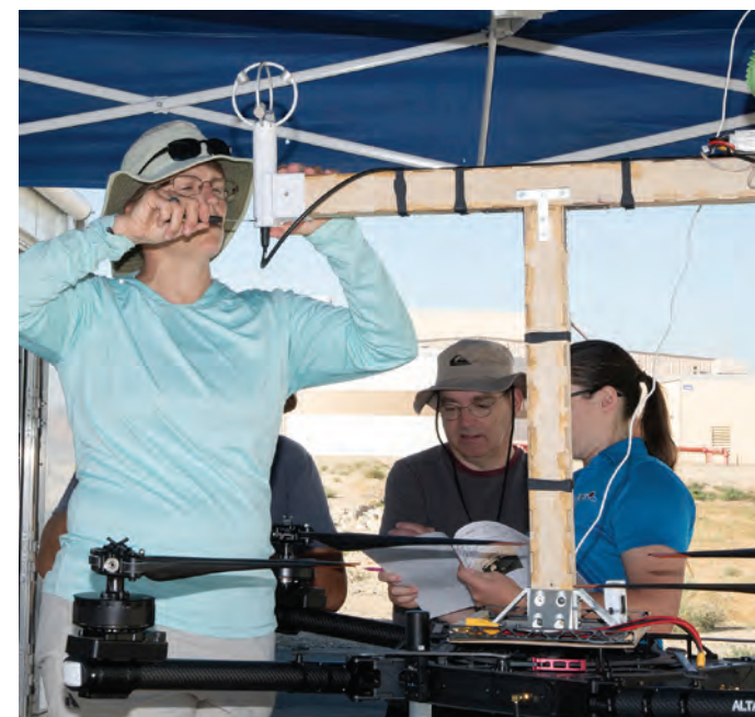
(left) Researchers work on securing sensors onto the test fixture on the Alta-X aircraft. (right) The Alta-X aircraft flies at NASA's Armstrong Flight Research Center in Edwards, California, as part of the AEROcAST campaign.
