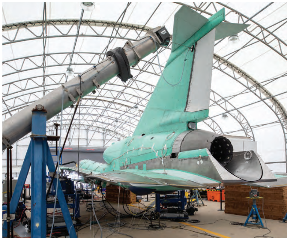
The X-59 aircraft undergoes ground vibration testing at Lockheed Martin's Palmdale facility.
