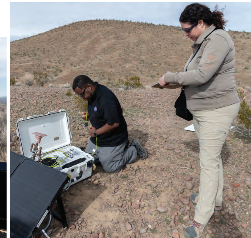
The Carpet Determination In Entirety Measurements (CarpetDIEM) Phase III flight campaign deployed and tested a state-of-the-art ground recording system and autonomous triggering technology.
