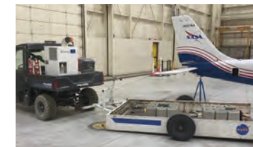
The aircraft testing setup with batteries on tow cart.
