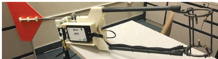
SonicSonde concept illustration and sensor suite in the lab (left). Full deployment field test and close-up of sensor suite tethered to cable line (right).
