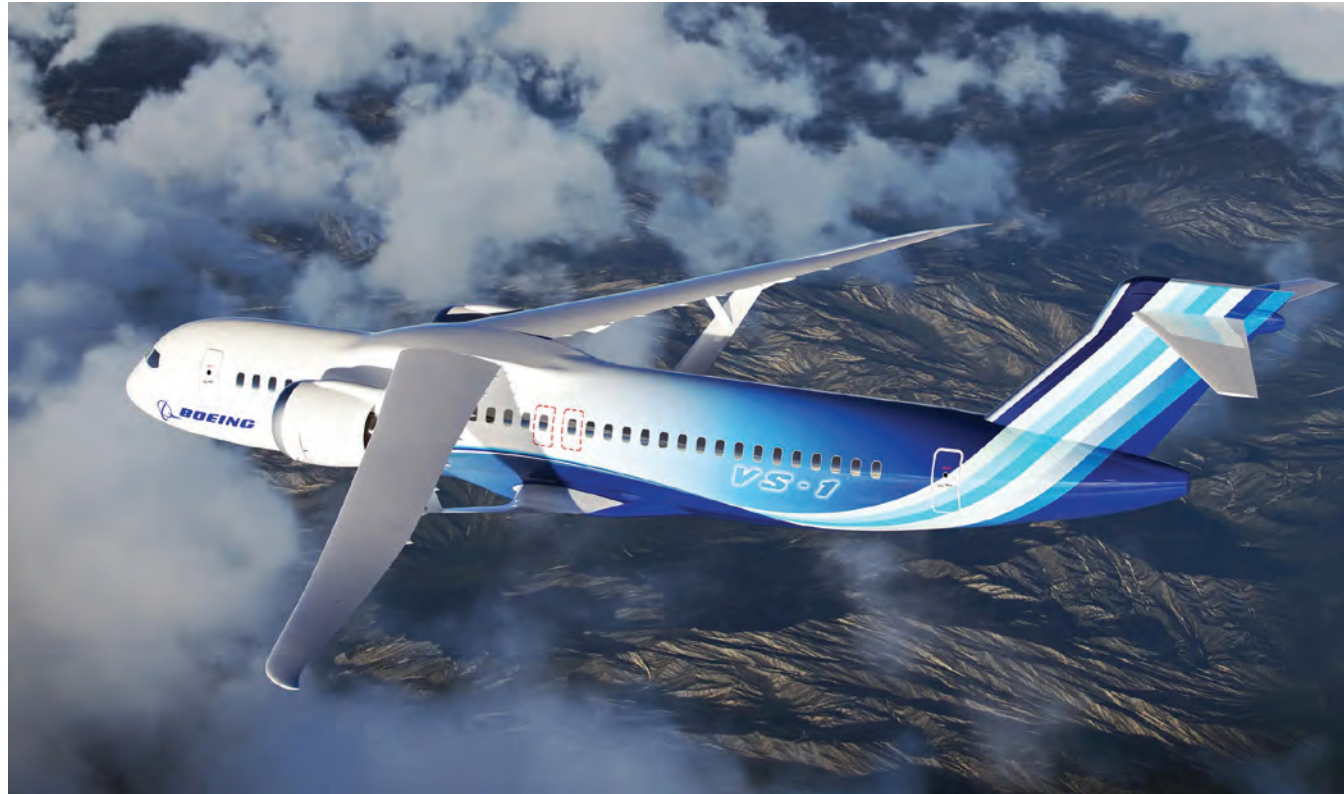
Artists concept of the Transonic Truss-Braced Wing Airplane with geometrically nonlinear wing deformation. Credits: Boeing
