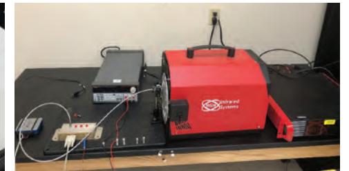
ARMS system characterization utilizing the small blackbody.
