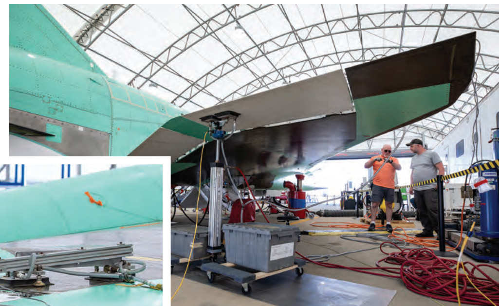
(below) The X-59 right aileron freeplay hardware.
