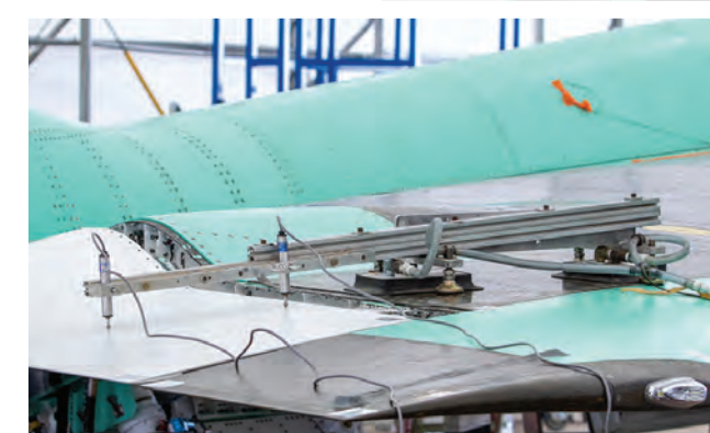
(below) The X-59 right aileron freeplay hardware.
