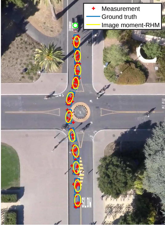
Figure 9: Illustration of the estimation results in a particular run by the proposed image moment-based RHM. The target is initialized as a circle (green circle) with a radius of 20 pixels. The estimated result (yellow ellipse), the measurements (red crosses) and the ground truth (blue box) are shown for every 40 frames.
