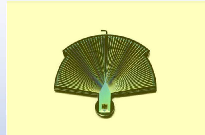
NASA JPL's new single-photon detector comprises 32 superconducting nanowires
