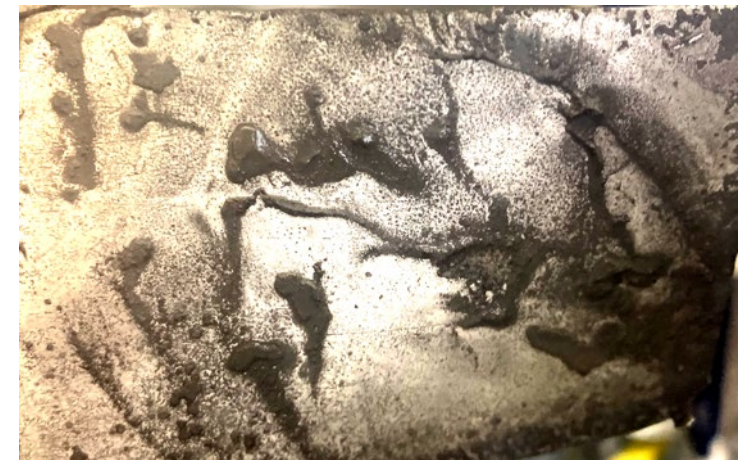
Anode surface at end of life
