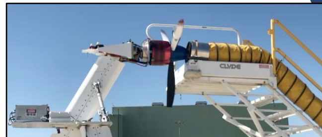
Airvolt static propeller test stand with cooling duct
