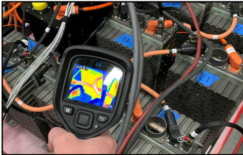
Battery Module Thermal Performance during Mission Profile Load Test
