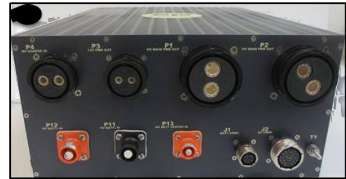
Battery Control Module (25 lb) contains BMS, contactors, HV distribution
