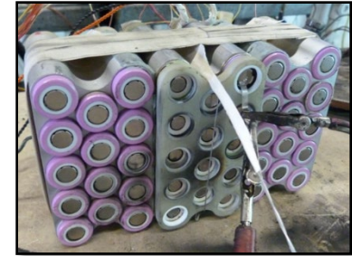
NASA JSC Test Unit With Interstitial Barrier and Heat Spreader (Design Template)
