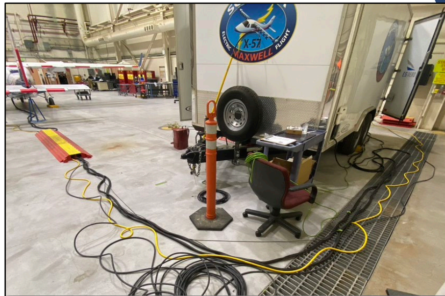
Ground Support Equipment “Battery Support System” charges, simulates, and tests aircraft traction batteries
