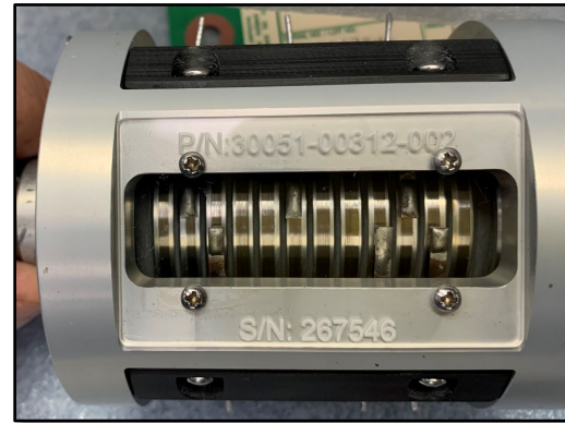
Slip Ring brush arms and rotor rings via inspection window Also visible: pins not in use after channel reassignment ("guard channels" providing extra clearance)
