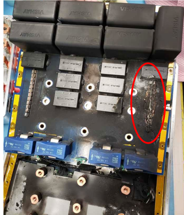
Flight XM3 CMC Row of Capacitors Failed due to Error in Assembly Process to Properly Isolate DC Bus and Gnd
