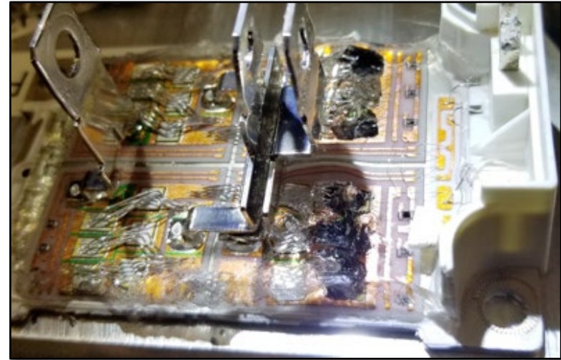
BM2 MOSFET Catastrophic Failure from Vibe
