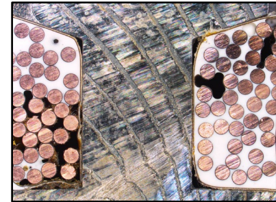
Improved fabrication process still exhibits some voids
