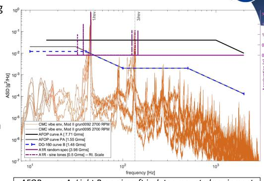
AFOP curve A: Light Prop aircraft isolator-mounted equipment AFOP curve PA: Transport aircraft isolator-mounted equipment DO-160 curve B: Fixed-wing Turbofan equipment rack
