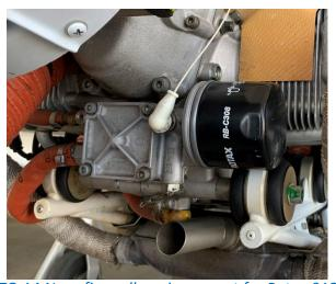
TG-14 Nose firewall engine mount for Rotax 912
