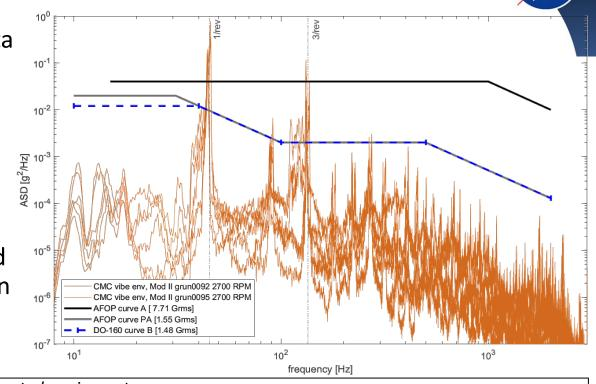
AFOP curve A: Light Prop aircraft isolator-mounted equipment AFOP curve PA: Transport aircraft isolator-mounted equipment
