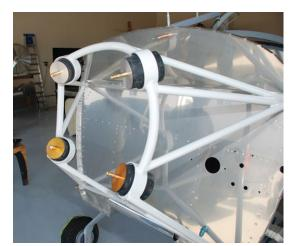
Nose firewall engine mount for IO-360
