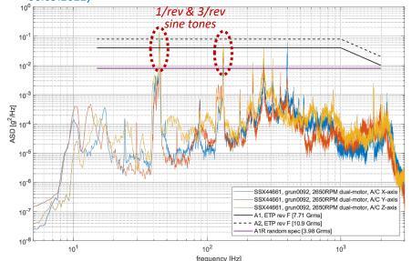
Right upper mounting rail data (09.27.2022), full-fine prop pitch dual motor run. Right motor balanced to 0.04 IPS (NAMIS WR D-0200895 on 04.28.2022).
