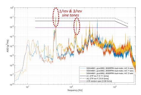
Left CMC data (09.01.2022), full-fine prop pitch dual motor run Left motor balanced to 0.03 IPS (NAMIS WR D-0220678 on 06.09.2022) Installed-isolator stiffness provides damping >200 Hz
