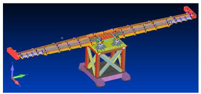
Yellow dots with coordinate systems represent where instrumentation was placed on the test article during modal testing
