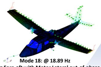
Wing Fore-aft with Motor Lateral out-of-phase
