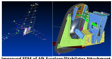
Improved FEM of Aft-fuselage/Stabilator Attachment
