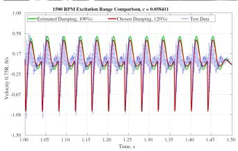
Measured aerodynamic and friction damping for HL propeller by exciting blade folding mechanism using pulses of compressed air.
