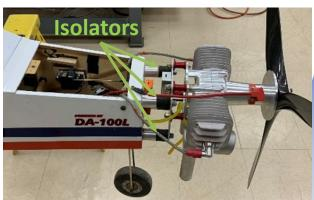
AFRC Model Lab aircraft motor with 4 corner- mounted isolators
