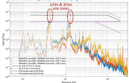
Right CMC data (09.27.2022), full-fine prop pitch dual motor run Right motor balanced to 0.04 IPS (NAMIS WR D-0200895 on 04.28.2022) Installed-isolator stiffness provides damping >90 Hz
