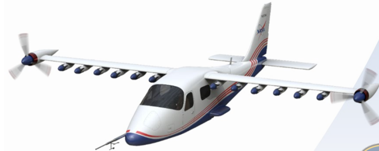
X-57 Mod IV in High-Speed (Cruise) Configuration
