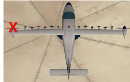
DiTTo Cruise Motor Failure (Cruise Fail)
