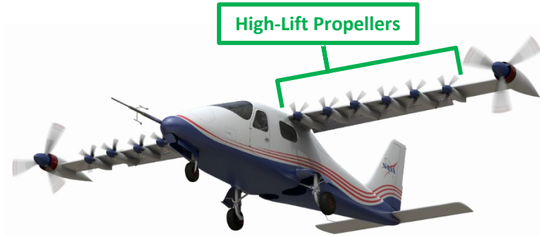
X-57 Mod IV in Low-Speed (Takeoff/Landing) Configuration
