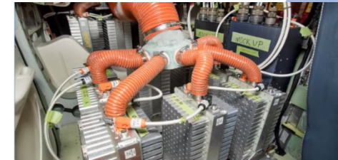
Battery Venting (3" dia)
