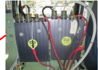
Battery Venting Assembly
