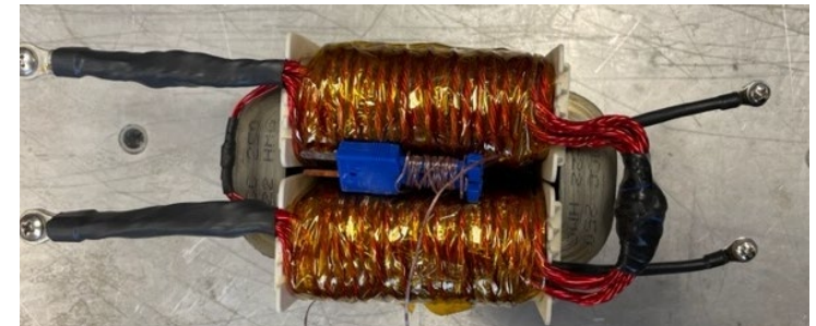
3.3 kVA single-phase design (3x for 10 kW)
