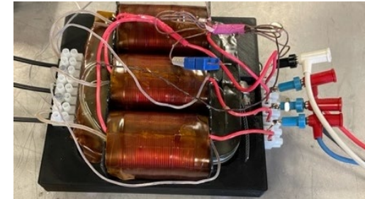
3.3 kVA single-phase design (3x for 10 kW)
