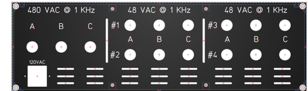
NASA 1 kVA 3-phase design
