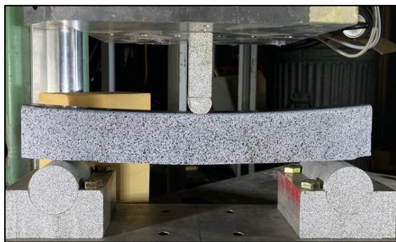
Figure 3. Three-Point Bend Test Setup
