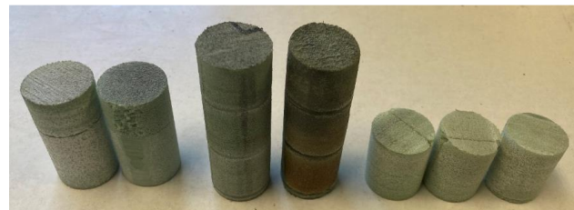
Figure 6. Foam-only plugs isolated from as-fabricated specimens.
