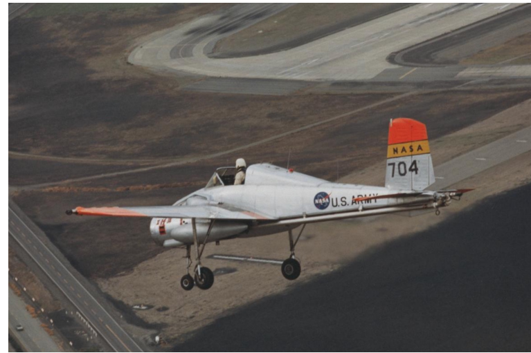
Bell X-14B (VTOL experimental aircraft)
