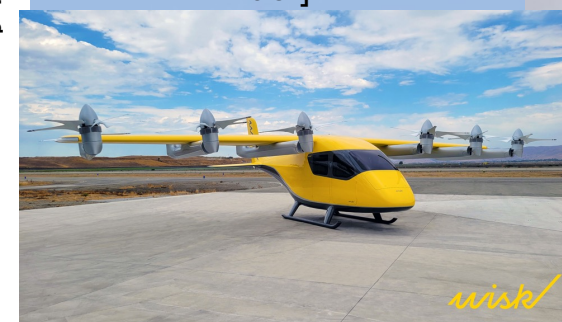
Wisk Cora (Lift + Cruise, tilt rotor Hybrid)
