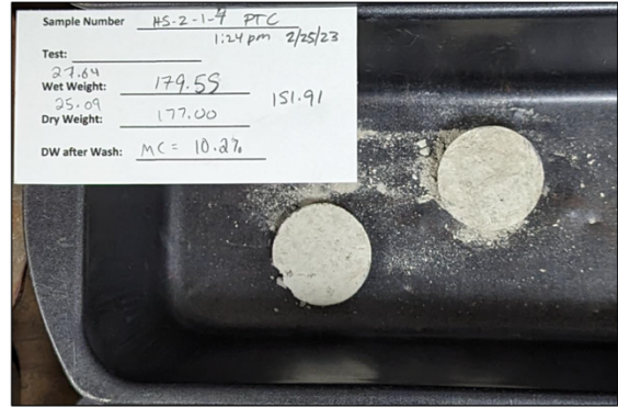
Figure 4-2. Example of a UTTR Surface Crust Direct Shear Test
