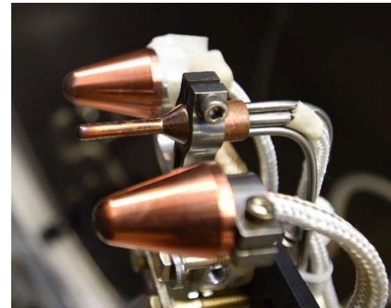
Trident sweep arm with water-cooled sensors
