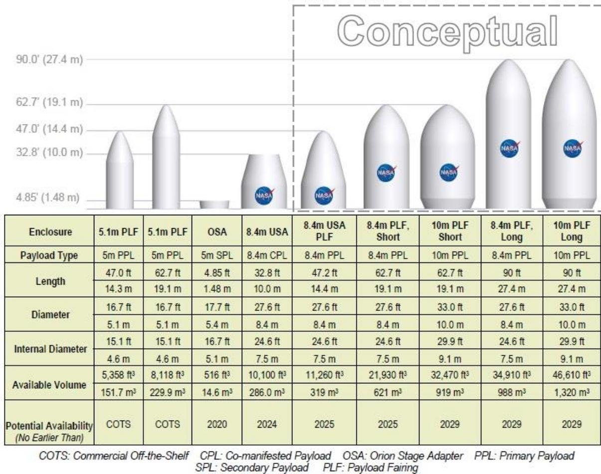
**Figure 3: SLS payload fairing options.**
