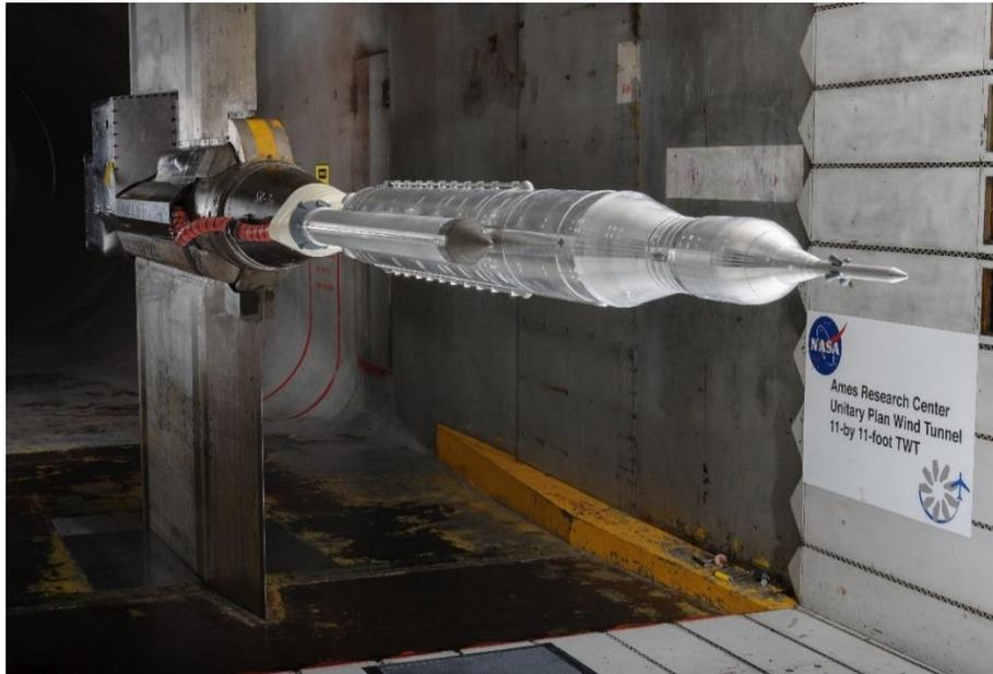
**Figure 4: Wind tunnel testing of SLS Block 1.**
