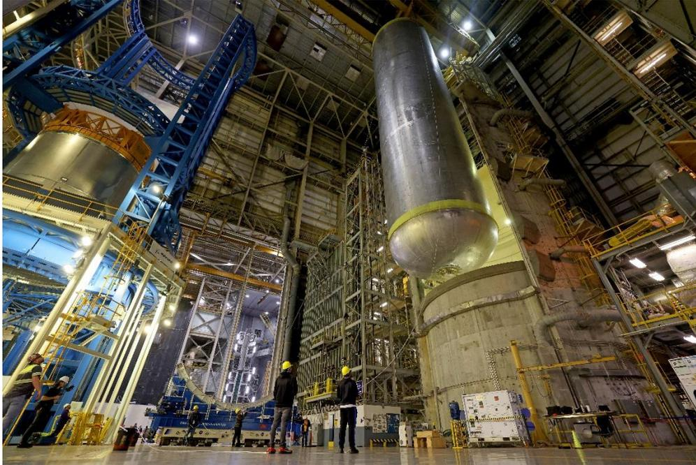
**Figure 7: Technicians finished welding the 51-foot Artemis III liquid oxygen tank structure, left, inside the Vertical Assembly Building at NASA's Michoud Assembly Facility in New Orleans Jan. 8, 2024. The Artemis III liquid hydrogen tank, right, completed internal cleaning Nov. 14, 2023.**
