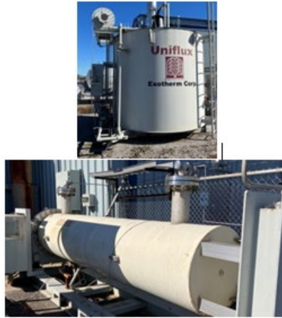
Figure 13. Heaters for Hot-Gas Valve and Propellant Tank Diffuser Testing
