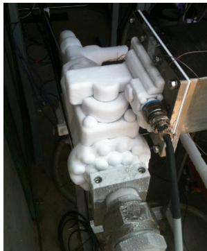
Figure 11. Cryogenic Valve Flow Testing
