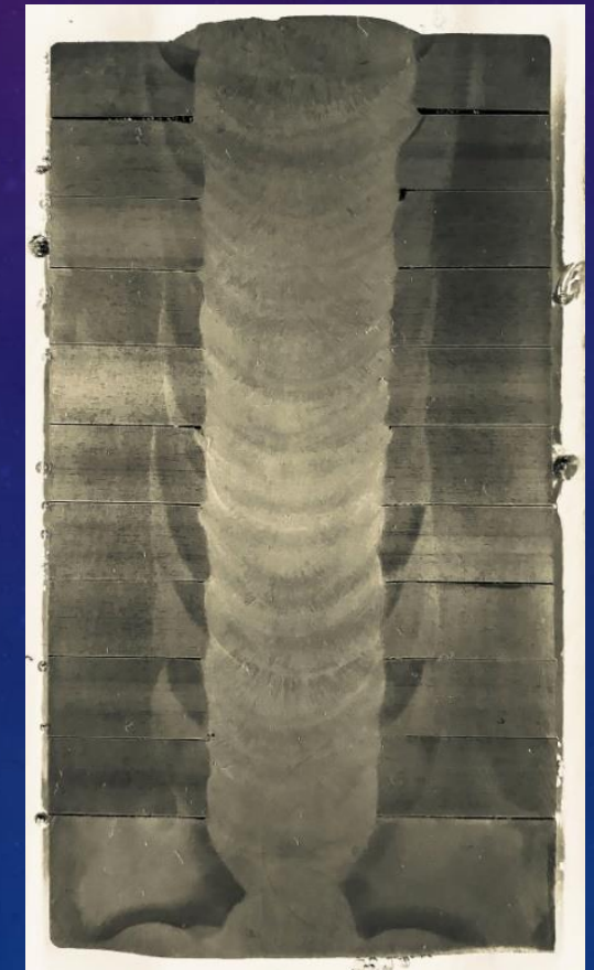
Shell to shell weld cross section
