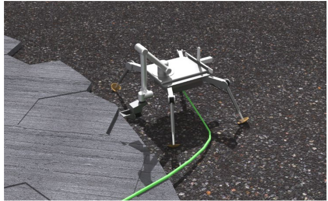
Fig. 4 MMPACT Arm and Platform Constructing Landing Pad
