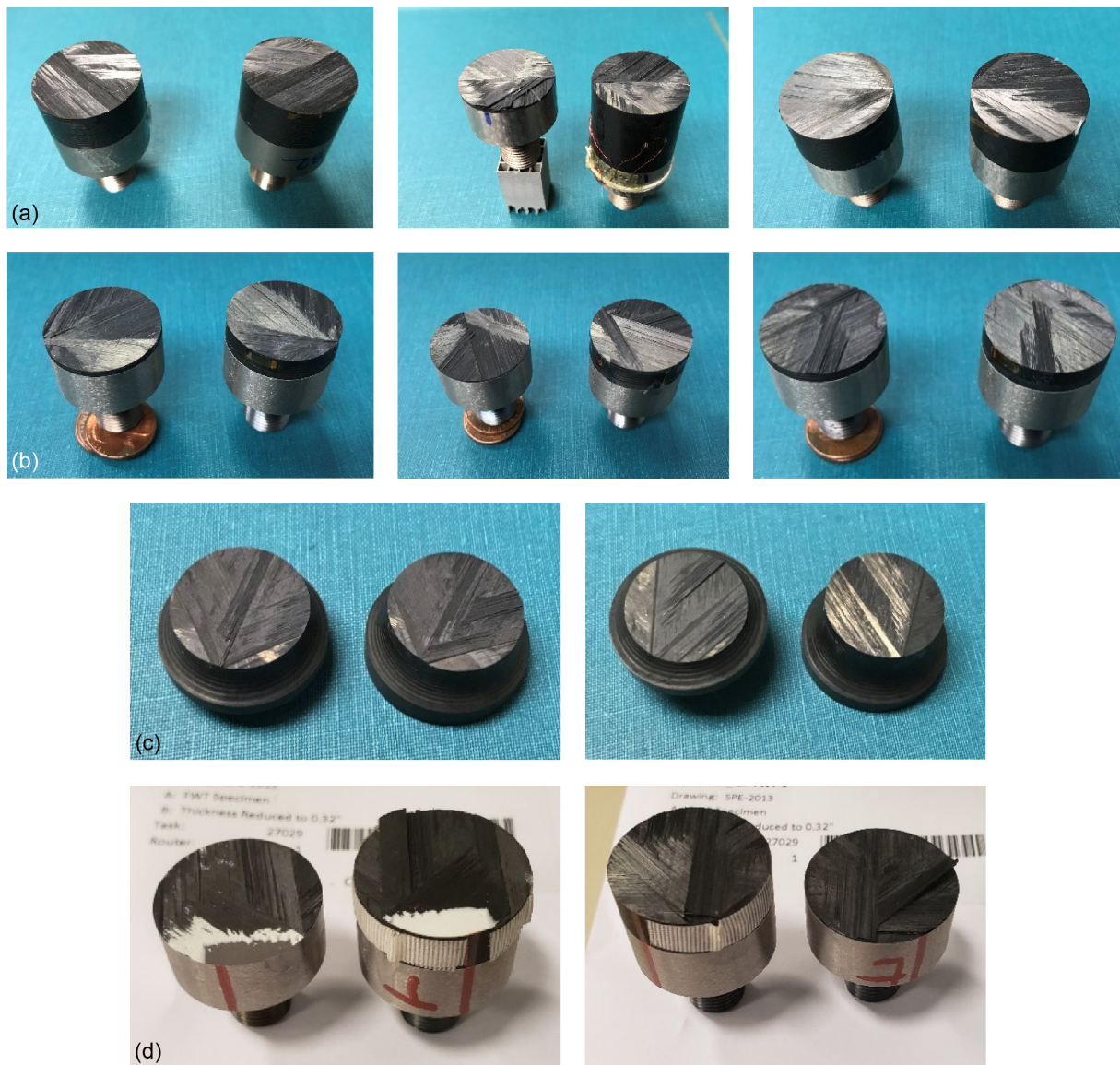
Figure 6.—Example fracture surfaces of baseline test specimens. Nominal specimen diameter is 1 in. (a) Thick. (b) Thin, radiused. (c) Spool. (d) Thin, straight-sided.
