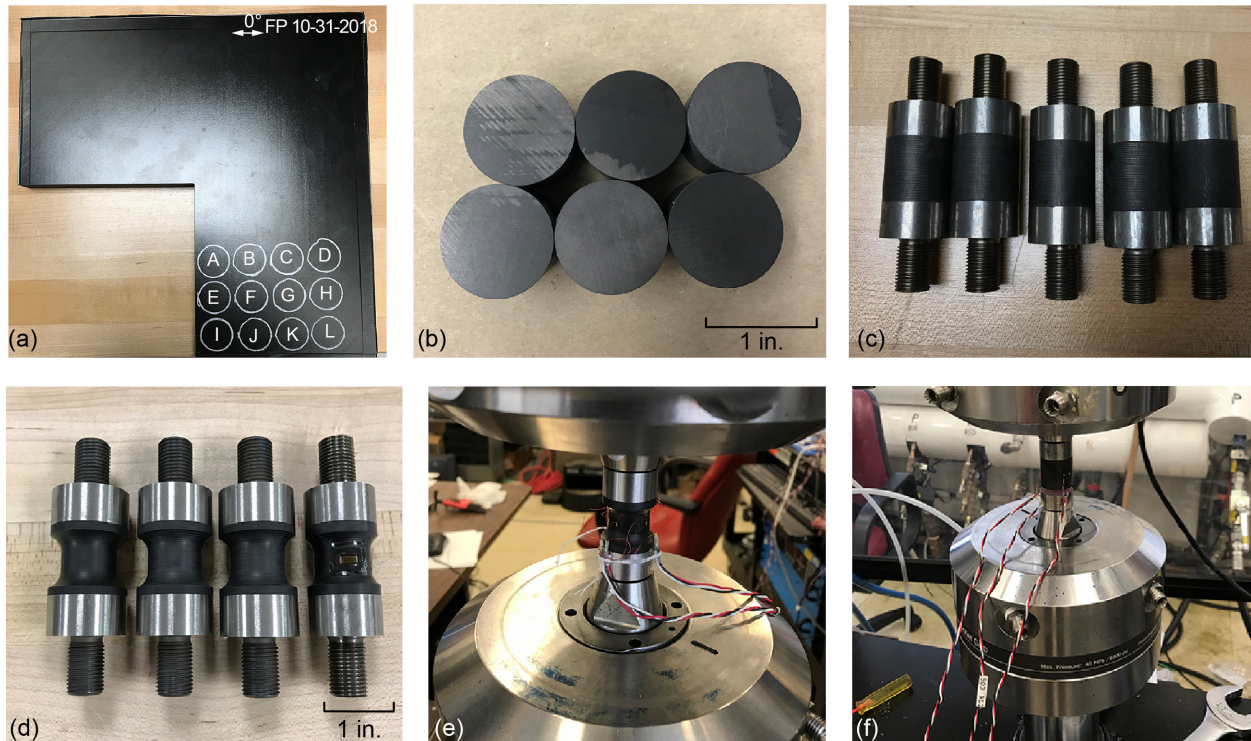
Figure 2.—Stages of specimen production and testing. (a) Starting plate with cutting layout. (b) Cored specimens with faces ground parallel. (c) Specimens bonded to tabs and turned concentric. (d) Spool gage section cut into straight-sided specimens. (e) and (f) Strain gaged specimens mounted in the test rig. Pull-tab diameter is nominally 1 in.
