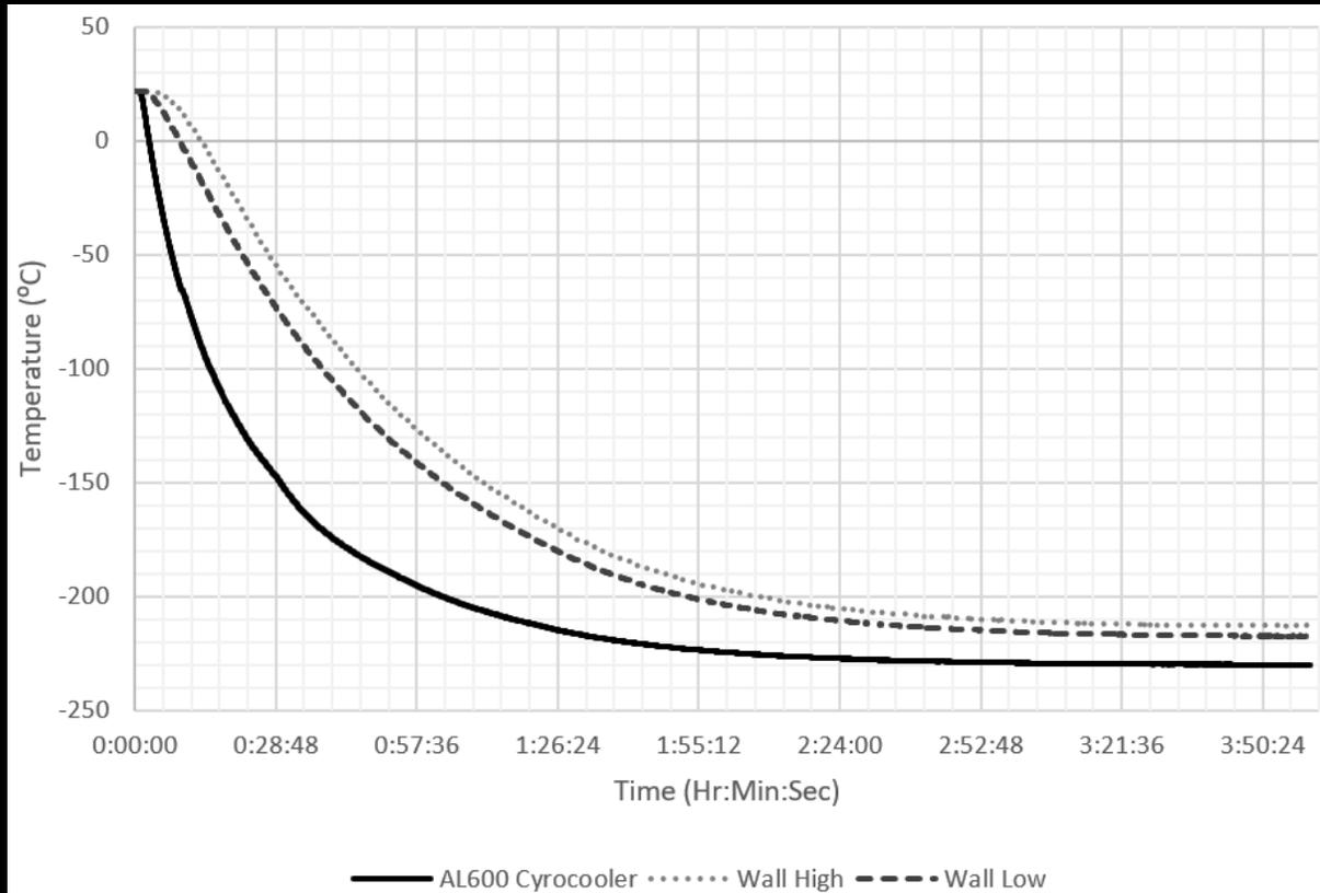
Cooldown performance prior to print. Temperatures typically increased to -190 ° C during printing due to extruder and print heat.
