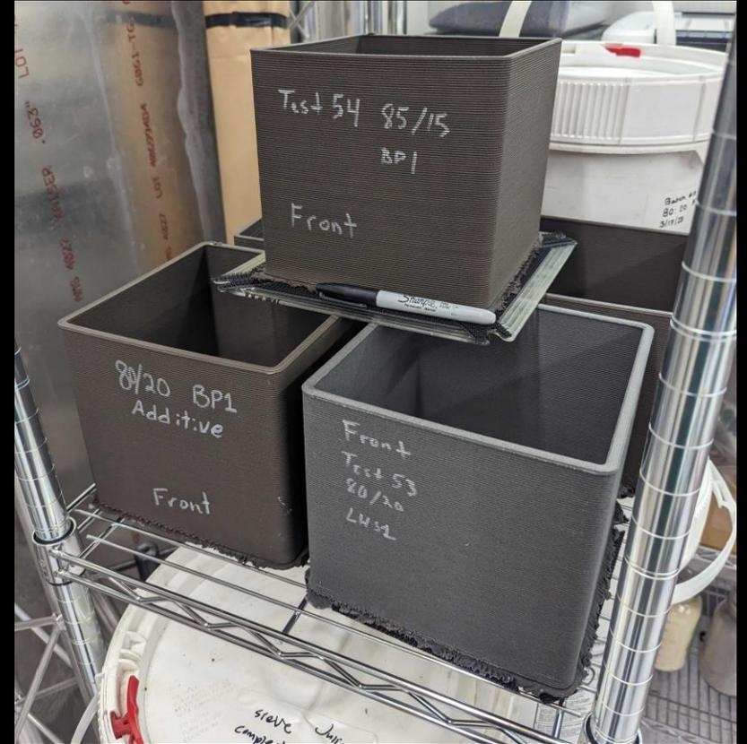
Printed test samples prior to water-jetting
