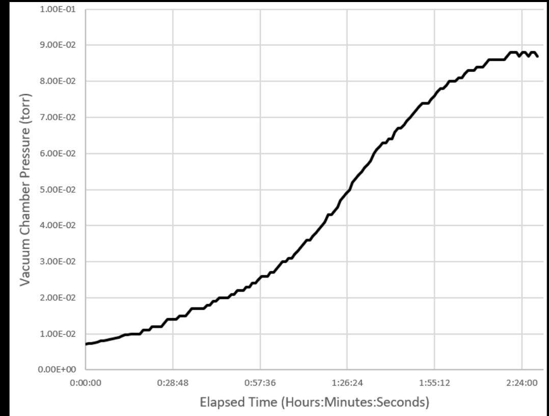
Vacuum performance during print. Pressure increase is likely due to water sublimation off the thermal shroud when warmed by the extruder and print.
