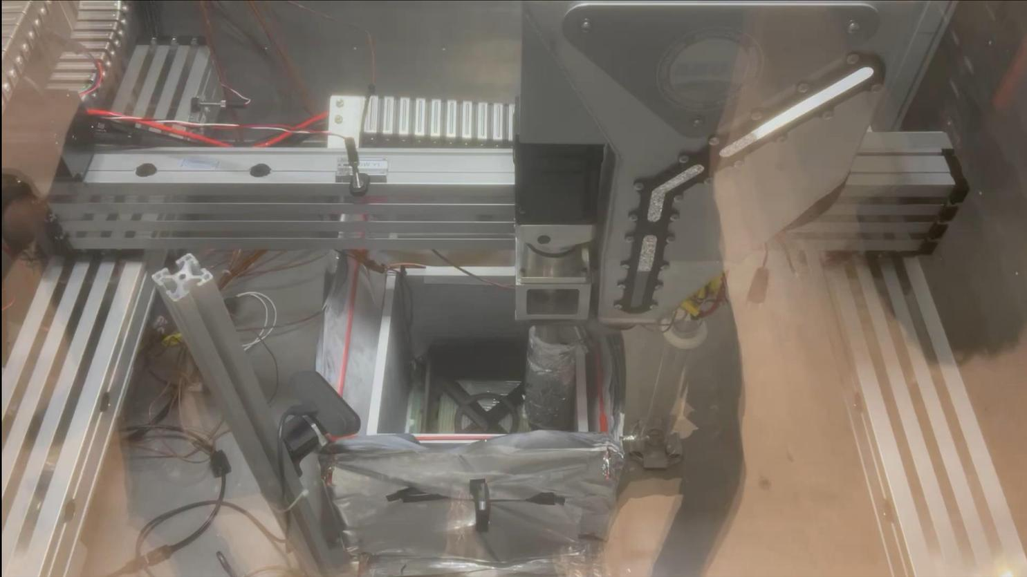
Test samples are printed in TVAC. A thermal shroud was kept below -190C. Vacuum pressure started at  $\sim 10^{-3}$  torr ends at  $\sim 0.8$  torr likely due to water sublimation off the shroud when warmed by the extruder and printed structure
