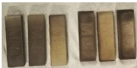
Figure 6. Discolored Madidrop tablets after wetting and drying.
