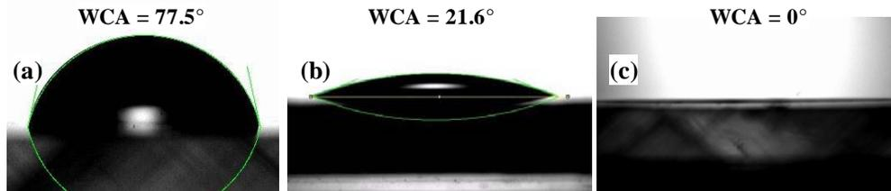
**Figure 8. WCA measurements. a) Uncoated polycarbonate. b) DLC with no plasma pretreatment. c) DLC with plasma pretreatment.**
