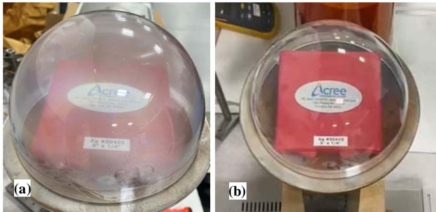
**Figure 16. Pictures showing results of fogging tests on (a) uncoated polycarbonate dome and (b) SHPL-DLC anti-fogging coated dome. Note that there is no fogging on the coated dome.**
