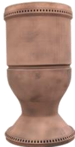
Selective Laser Melting (SLM) of GRCop-84
