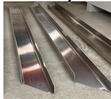
Brake-formed C-channel floor beams
