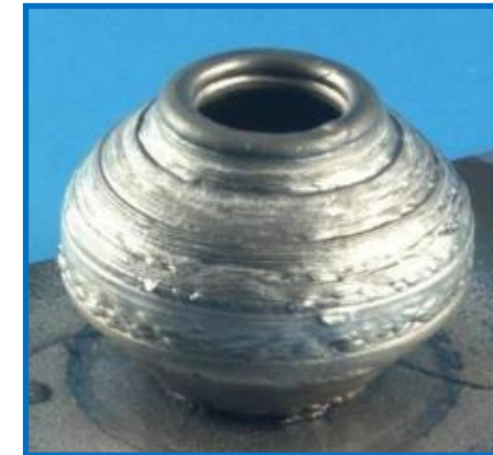
Build up part, layer-by-layer
