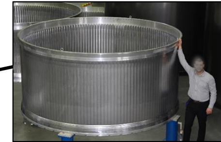
Flow-formed integrally stiffened skin and stringer fuselage
