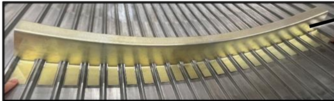
Stretch-formed Z-ring frames and shear clips
