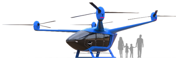
Figure 2: NASA quadrotor RVLT reference vehicle configuration considered in this study.
