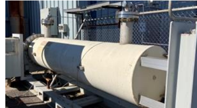
Figure 13. Heaters for Hot-Gas Valve and Propellant Tank Diffuser Testing
