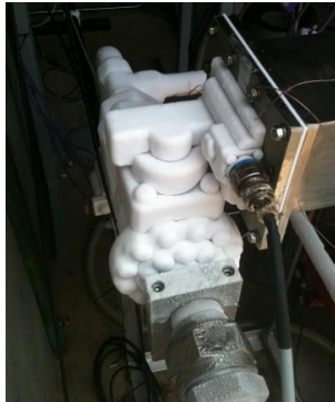
Figure 11. Cryogenic Valve Flow Testing
