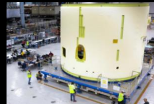
Liquid oxygen tank manufactured
