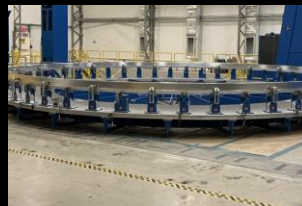
Interstage structural test article aft L-ring on Ingersoll Machine
