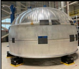
Exploration upper stage LOX dome weld confidence article
