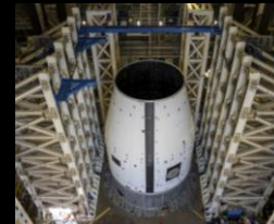
Universal stage adapter development test article in test stand at NASA Marshall
