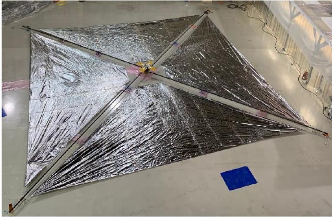
Figure 2: Solar Sail fully deployed at the test facility at NASA Langley Research Center [6].
