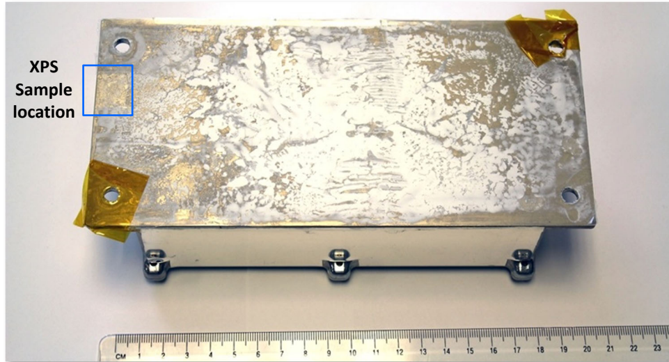
Figure 67. The bottom side of the MISSE 8 SEUXSE Power Box showing the white Nusil CV-9341 thermally conductive silicone grease that was applied pre-flight.
