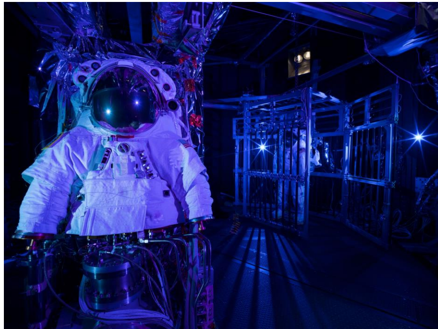
Figure 3. Setup of the government reference xEMU TVAC test. (Image by NASA)
